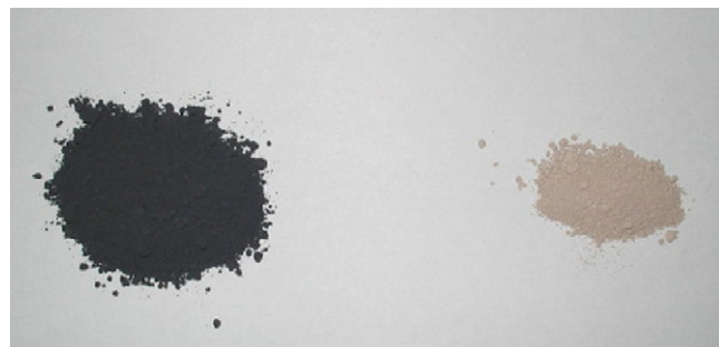
Fig. 2. The color change of GS by heat treatment. Left and right: before and after heating at around 923 K, respectively.
